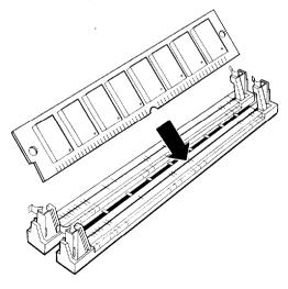
4. Push the SIMM into the socket until it is seated firmly in the slot. Then tilt it upright, as shown below, guiding the hole at each end of the SIMM over the retaining post at each end of the SIMM socket.
